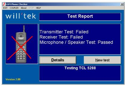
8 The subsequent Test Report shows you which test, if any, failed and invites you to view the results in more detail.
