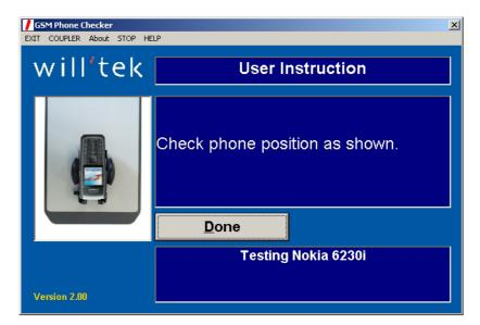
5 Follow the instructions on the screen, if the GSM Phone Checker Software proposes further action (e.g. adjusting the phone on the cradle or pulling out the antenna).
