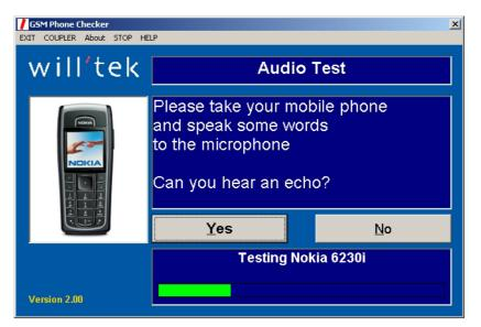
6 For the audio test, speak into the mobile's microphone and check if you can hear your voice in the speaker after one or two seconds. You can lift the phone from the antenna coupler, however, do not move it more than half a meter (1.5 feet) away from the coupler.
