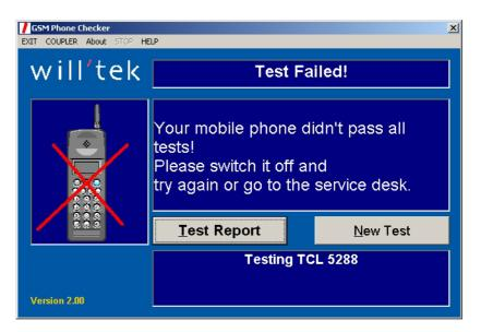
7 After completing the tests, the GSM Phone Checker Software presents a pass or fail indication and allows you to check the test report or start a new test. Select **Test Report** to view the test results, or select **New Test** to return to the start menu for another test.
