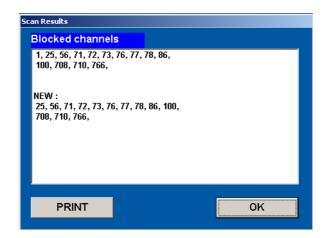
8 If you are not using a mobile phone covering all frequency bands that you need to test, repeat the scan procedure with another phone supporting the remaining band(s). Do not clear the previously generated channel list in the second run but select **Search more** instead.
